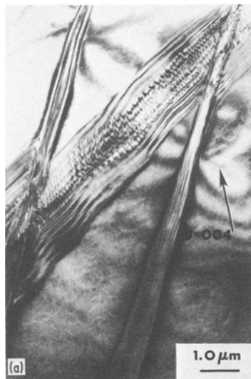
Figure 5 Bright-field electron micrographs of Type I precipitates formed at 1000^{\circ}\text{C} for 1 h. Imaging with the several g -vectors shown confirms that the habit plane is \{311\} . Note that g \cdot R = 0 for two of the precipitates imaged with g = 044 .
